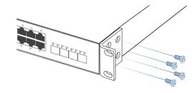
② Secure the mounting brackets to an EIA standard size (19") rack.
